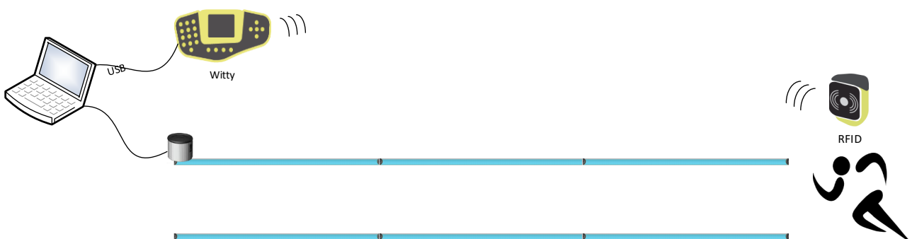
Figure 107 - Witty RFID communicates by radio through a Witty Timer with USB attachment
