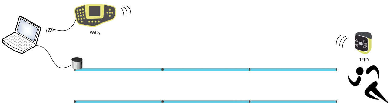
Figure 111 - Witty RFID communicates by radio through a Witty Timer with USB attachment
